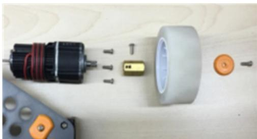
(A) Connect the motor and the wheels
