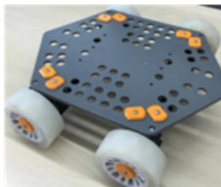
(B) Fix the wheel to the chassis
