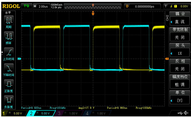
FIG. 11. SIMO driving voltage waveform of switch and (yellow line: the waveform of S_1 ; blue line: the waveform of S_2 ).
